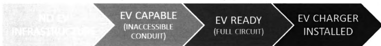
Figure 1: Four Levels of EV Charging Readiness
