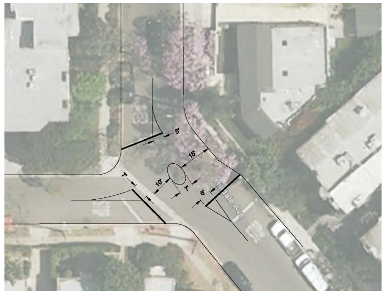
Figure 10. Preliminary Design of the Traffic Circle at Hilldale Avenue & Vista Grande Street
