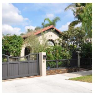
☑ Driveway gates located within the front setback should be low, or have open elements for the upper portion.
