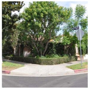
☑ On corner lot properties, consider locating fences or walls at a diagonal across the corner to eliminate blind corners for pedestrians on the sidewalk.
