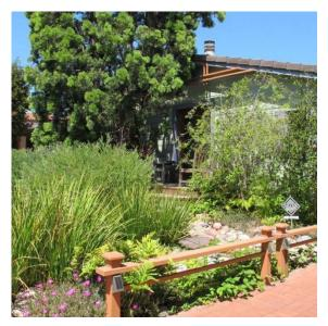
☑ Consider natural drainage patterns when locating features and structures. Here, a cobble swale directs stormwater through the landscape.
