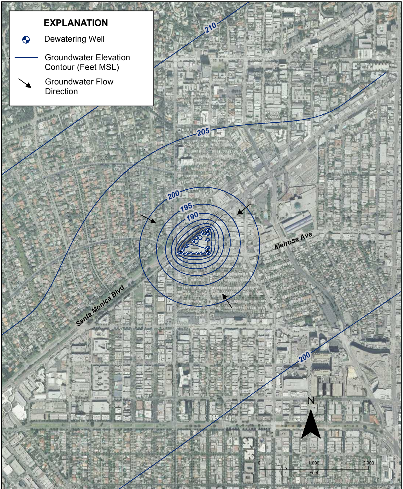
Simulated Regional Groundwater Elevation Contours During Dewatering Phase - Model Scenario 5 Proposed Melrose Triangle Development Corners of Santa Monica, Melrose, & Almont West Hollywood, California
