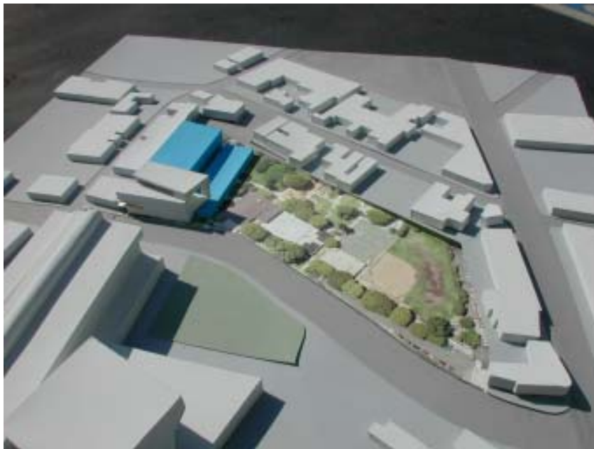
The Library. The library will be built on the site of the existing Ron Stone Clinic. Vehicular access to the freestanding parking structure is accommodated through the ground floor level of the library from San Vicente. The library's 90-car garage is built to the north of the free standing structure and becomes the plinth upon which the south end of the park sits, thus leveling the topography of the park and expanding its useful area..
