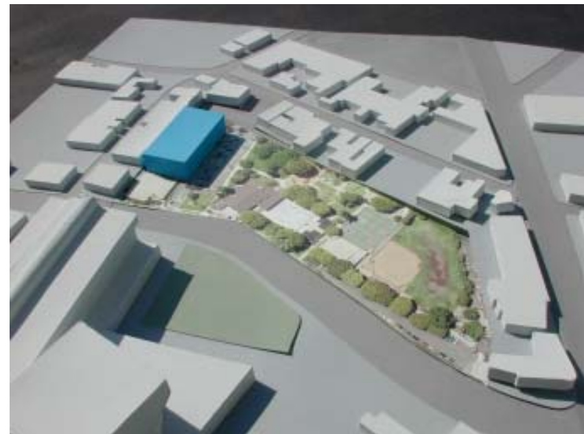
Freestanding Parking Structure. The new structure will fit behind the existing Ron Stone Clinic building on the site of the Ron Stone parking lot, the tennis courts and the El Tovar Maintenance Yard. The tennis courts will be replaced on the roof of the new structure.
