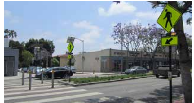
Rapid Flashing Beacons, Santa Monica Blvd.
