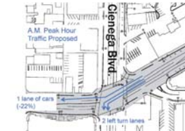
Remove bottleneck by shifting transition east of La Cienega: existing above; proposed below.
