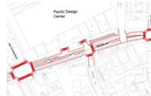
Remove bottleneck by eliminating one-block long additional lane: existing above; proposed below.
