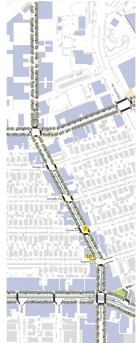
Proposed improvement plan for the entire street showing curbside parking, wider sidewalks, curb extensions with directional ramps, street trees in planted tree wells and street lights..
