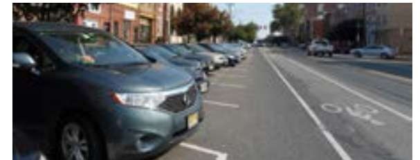
Pictured: Backed-in angled parking provides enhanced safety, visibility, and comfort for bicyclists, drivers, and pedestrians.
