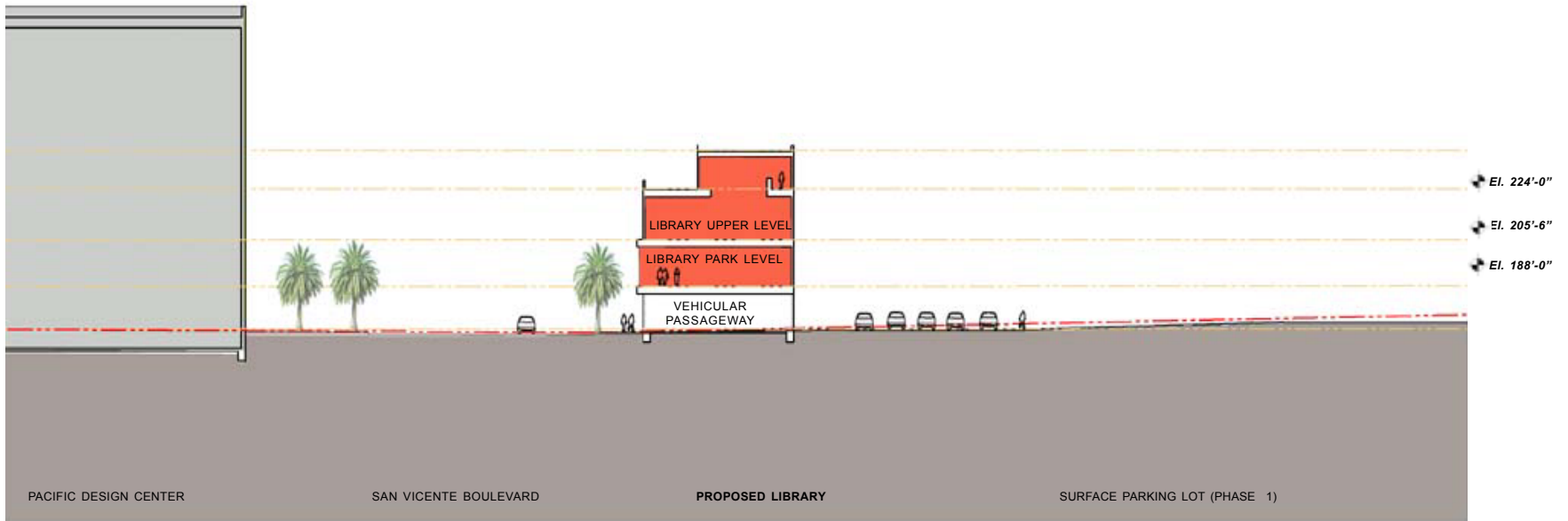
East-West Site Section Through Library Looking South
